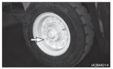
Install steer wheel. Put two nuts opposite (180°) each other. Tighten both. Install remaining nuts. Tighten all nuts in a sequence opposite (180°) each other. Tighten to 440+35 N·m (325+25 lb-ft).
