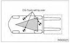
For the lift truck to be stable (not tip over forward or to the side), the CG must stay within the area of the lift truck stability base - a triangular area between the front wheels and the pivot of the steer wheels. If the CG moves forward of the front axle, the lift truck will tip forward. If the CG moves outside of the line on either side of the stability base, the lift truck will tip to the side.
