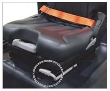
16. To position the seat, PUSH the lever away from the seat track and move the seat forward or backward to a comfortable position.
