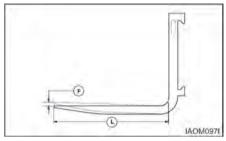
Check the difference in height of one fork tip to the other when mounted on the fork carrier. A difference in fork tip height can result in uneven support of the load and cause problems with entering loads.
