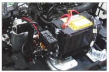
Remove the front cover from the box. The fuses are in the box.
