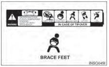
Spread your legs wide and secure the feet to the inner sides of the compartment.
