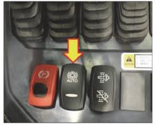
This switch is used to select auto/manual shift on the gearshift.
