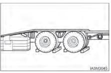
Always block the trailer or the rail car wheels before loading the lift truck.
