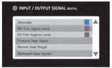
The vehicle digital signal can be checked (Alternator, RH turn signal lamp, LH turn siganal lamp, forward gear signal, neutral gear singal, Backward gear singal)
