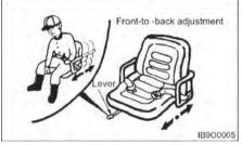
Move the lover, slide the seat to the desired position, and release the lever.
