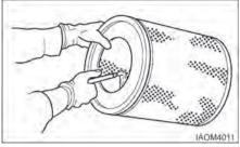
Direct water on the inside and outside of the element along the length of the pleats. Air dry it thoroughly and then examine it.
