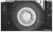
Install drive wheel. Put two nuts opposite (180°) each other. Tighten both.
