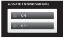
This safety function enables operation only when the seat is occupied and the safety belt is on.
