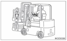
Tilt elevated load forward only when directly over unloading area and with load as low as possible.
