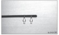
The oil level should be close as possible to upper point of the oil dip stick. Do not refill more than upper point.
