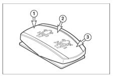
Press this switch and release it after 3 sec, SCR Cleaning will be started and the engine speed will be increased. Screen pop-up provides information on the warning up and cleaning process.
