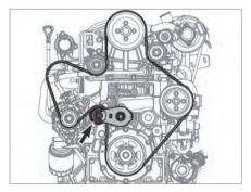
Inspecting the condition Inspect the Micro V-belt for cracks, oil, overheating and wear.
