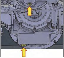
1. Remove the drain plug, spring and strainer. Allow the oil to drain.
