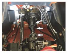
3. Lubricate the grease into the nipples of the universal joint.
