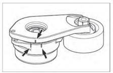
The vertical rod shown by the arrow is the "pointer," and the belt replacement period is indicated when this "Pointer" enters the horizontal range shown in orange.
