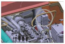
13. Observe the engine coolant level in the coolant recovery bottle. With the engine cold, maintain the level to the COLD mark. If the recovery bottle is empty, also fill the radiator at the top tank.
