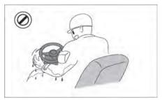
Never operate a lift truck with wet hands or shoes. Never hold any controls with grease on your hands. Your hands or feet will slide off of the controls and cause an accident.
