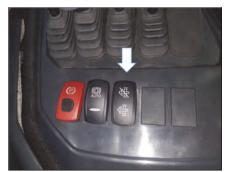
This switch initiates regular regeneration process of the post-treatment device.
