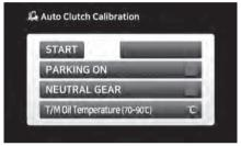
After any service below, should conduct the auto clutch calibration. See the topic, "Drive axle Oil, Transmission Oil, Oil Filter & Strainer - Clean, Change" in First 50-100 Service hours or a week.
