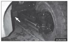
Inspect the suspension mounting bolts. Tighten suspension mounting bolts, if necessary, to 240±30 N·m (180±20 lb-ft).
