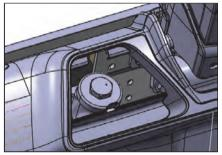
The brake reservoir is located on the left side of the steering column.
