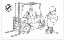
Forklift trucks may only be refueled at specially reserved locations. Switch off the engine when refueling. Smoking and handling of naked flames during refueling are strictly prohibited. This prohibition also applies during the changing of the LPG (liquefied propane gas) tank. Mop up spilt fuel and do not forget to close the fuel tank before restarting the engine.
