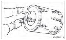
Direct air on the inside and outside of the element along the length of the pleats. Check the element for any tears, rips or damage.
