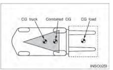
The stability of the lift truck is determined by the location of its CG; or, if the truck is loaded, the combined CG of the truck and load. The lift truck has moving parts and, therefore, has a CG that moves. The CG moves forward or backward as the mast is tilted forward or backward. The CG moves up or down as the mast moves up or down. The CG and, therefore, the stability of the loaded lift truck, is affected by a number of factors such as:
