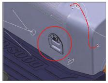
2. Pull the latch to raise the hood and seat assembly. Make certain the support cylinder will hold the hood open.
