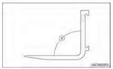
Check the angle between the upper face of the blade and the front face of the shank. The fork should be withdrawn from service if angle (C) exceeds 93 degrees or deviates by more than 3 degrees from an original angle other than 90 degrees, as may be found in some special application forks.
