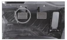
Inching Control Pedal - Pushing down the inching pedal, modulates the hydraulic pressure to the clutch packs, permitting disc slippage.
