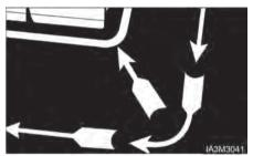
2. In narrow aisles, keep away from the stockpile when turning into the aisle. Allow for counterweight swing.
