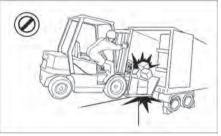
Do not operate on bridge plates unless they can support the weight of the truck and load.
