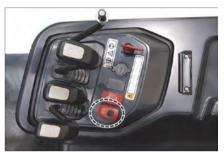
1. Engage the parking brake, if not already engaged. Place the transmission directional control lever in the NEUTRAL position.
