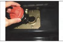
Remove the dipstick/ filter cap. Maintain the oil level to the FULL mark on the breather/dip stick.
