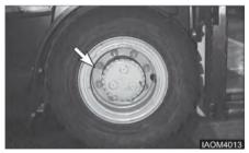
Do not reinflate a tire that has been run while flat or underinflated, without first checking to make sure the locking ring on the rim is not damaged and is in the correct position. When tires are changed, be sure to clean all rim parts and, if necessary, repaint to stop detrimental effects of corrosion. Sand blasting is recommended for removal of rust.
