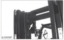
Inspect the part of the chain that is normally operated over the crosshead roller. When the chain bends over the roller, the movement of the parts against each other causes wears.
