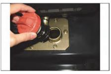
6. Stop the engine and check the oil level. With all cylinders retracted, maintain the oil level to the FULL mark on the dipstick.
