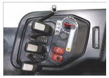
In case the lift truck is equipped with a electrical disconnect switch, the engine will not start unless the disconnect switch is in the ON (closed) position. Before starting, turn the disconnect switch to the OFF(open) position.
