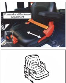
Adjust the seat before operating the lift truck. After adjusting, set the seat to make sure it is properly locked. Do not adjust the seat while the truck is in motion.
