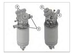
Install a new fuel filter and assemble the fuel filter cap.
