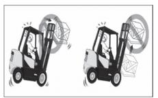
Do not elevate the load with the mast tilted forward. Do not tilt the elevated loads forwards. This will cause the lift truck to tip over forward.
