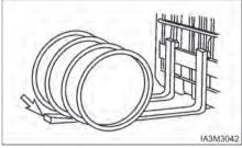
Block drums or round objects. Tilt the mast FORWARD and slide the fork tips along the floor to get under the load.
