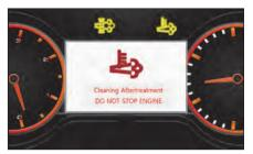
Display that notifies the operator of automatic SCR cleaning
