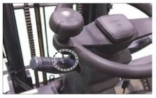
Select the direction of travel by pushing the directional lever FORWARD for forward direction or by pulling the lever BACK for reverse direction.
