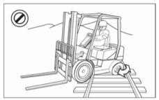
Do not go over rough terrain. If unavoidable, slow down. Cross railroad tracks slowly and diagonally whenever possible. A railroad crossing can give a loaded forklift truck a real jolt. For smoother crossing, cross the railroad diagonally so one wheel crosses at a time.
