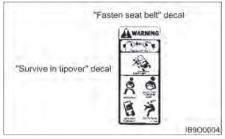
The "Survive in tipover" warning is located on the overhead guard. It shows the proper use of the operator restraint system.
