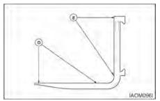
Check the straightness of the upper face of blade (D) and the front face of shank (E) with a straight edge.
