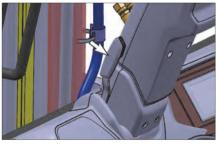
To adjust the steering column, push down the knob, and move the steering column to the desired position, then release the knob.
