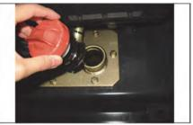
Raise the hood and seat assembly. Loosen the bolts of the hydraulic tank cover, and remove the hydraulic tank cover with filter assembly.
