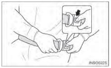
Push the button of the buckle to release the belt. The belt will automatically retract when released. Hold the plate of the belt and allow the belt to slowly retract.
