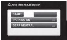
After any service below, should conduct the auto inching calibration. See the topic, "Drive axle Oil, Transmission Oil, Oil Filter & Strainer - Clean, Change" in First 50-100 Service hours or a week.
