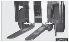
Raise the carriage high enough to gain access to the side thrust rollers on the back side of the carriage. Block the carriage in this position.
