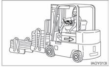
Use special care when operation on grades. Do not angle across or turn on grades. Do not use lift truck on slippery grades. Travel with forks downgrade when unloaded. Travel with load upgrade.
