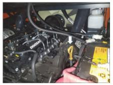
Measure the engine crankcase oil level with the dip stick. Maintain the oil level between the MAX. and MIN., (or FULL and ADD) notches on the dip stick.
