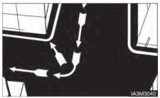
When turning sharp corners, keep close to the inside corner. Begin the turn when the inside drive wheel meets the corner.
