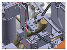
**Circuit Breaker** - Protects the main electrical circuits. To reset the circuit breaker, push the button in. It is located in the engine compartment.
