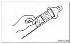
Belt Maintenance – Every 500 service hours. Check that the belt fastening works properly and that winding device is free from run lock when jerked. Check that the belt is suitably fastened to the seat. Check that the seat is correctly secured to the hood and the chassis. On visual inspection, fastenings must be intact, otherwise, contact the safety manager.
