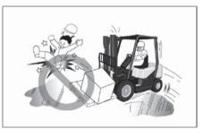
Do not drive on slippery surfaces. Sand, gravel, ice or mud can cause a tipover. If unavoidable, slow down.
