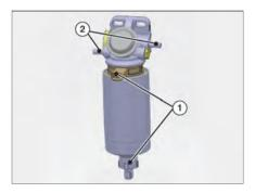
When removing the fuel filter, hold it carefully to prevent fuel from flowing out. Wipe and clean spilled fuel.
